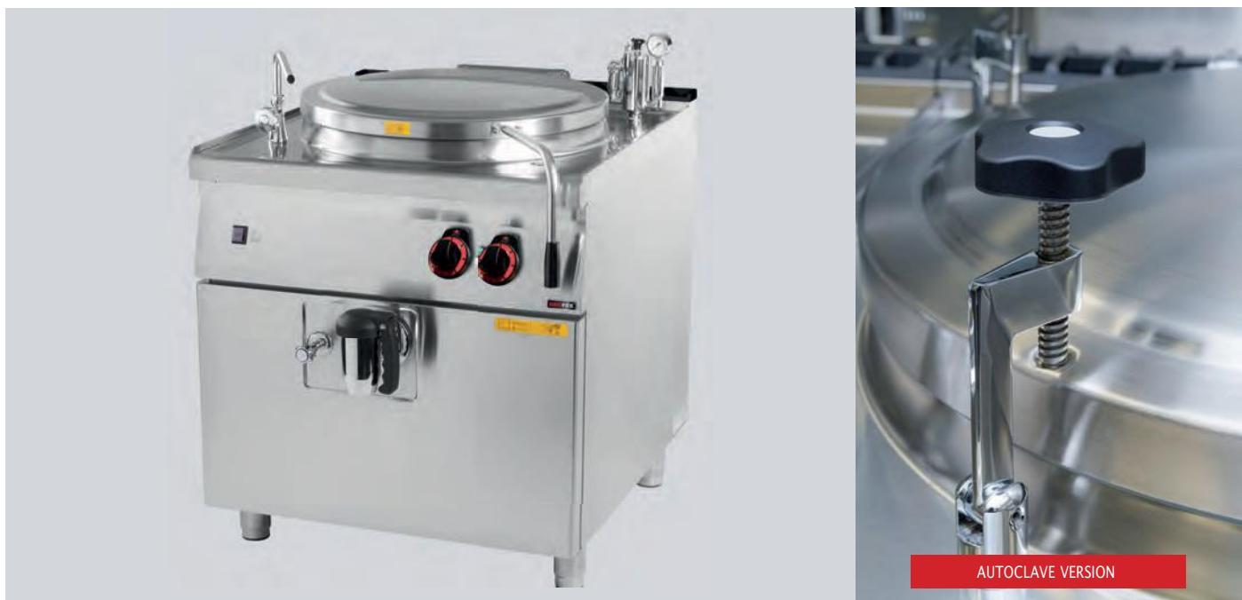
Bottom of tank made of AISI 316 (salt corrosion resistant, tank sides, top plate and front panel made of AISI 304. Thickness of material is 1,5 mm. Indirect heat in double-skin tank. Semi-automatic water filling system for easy and safe operation. Pressure controlled by safety-system gauge 0,5 bars and manometer. Conical seal available. Autoclave versions of all models for more efficient operation time and energy saving.
